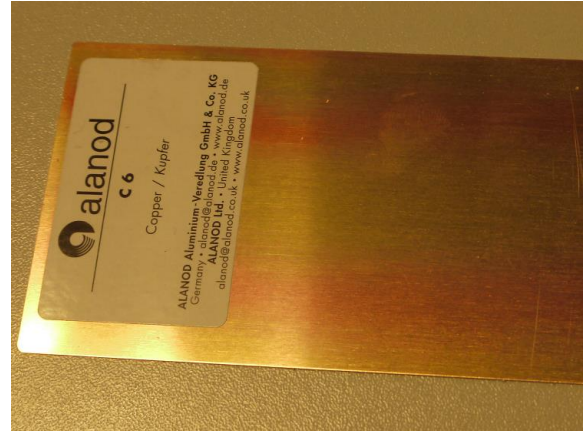
Figure 10. Photograph of the copper sample illuminated with fluorescence tube
