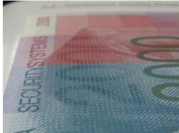
Figure 4. Intaglio latent image: Visible if the note is viewed at an oblique angle. The number 2000 appears in a light shade (viewing along the width of the note) or dark shade (viewing along the height of the note)
