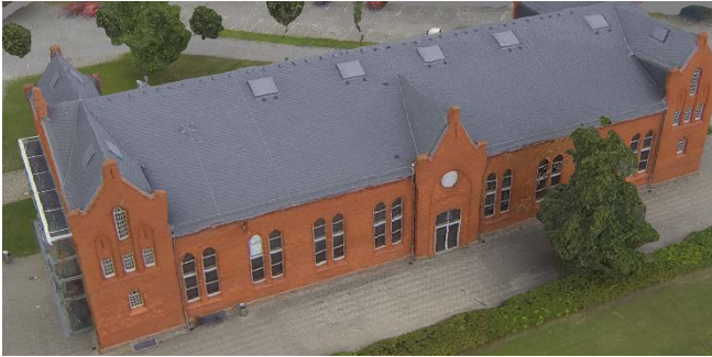
Figure 6. Reconstruction of the auditorium, textured mesh, with EXIF-data
