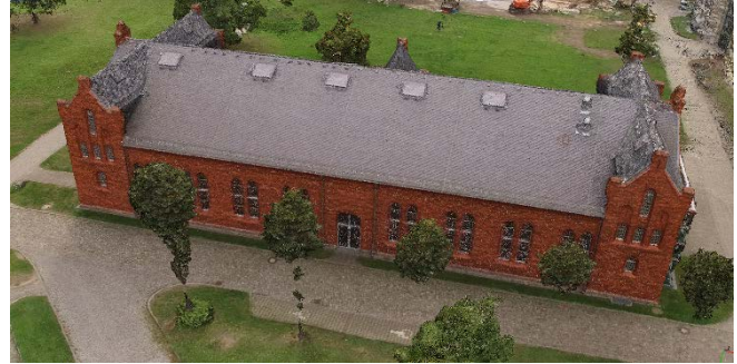
Figure 11. Reconstruction using 65 images (Dense Point Cloud)
