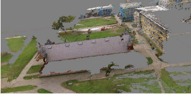
Figure 9. Reconstruction using 13 images (Dense Point Cloud)
