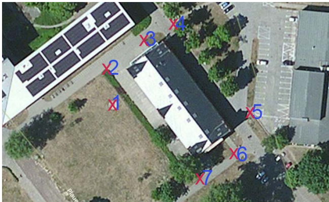
Figure 12. Selected Ground Control Points (GCPs)
