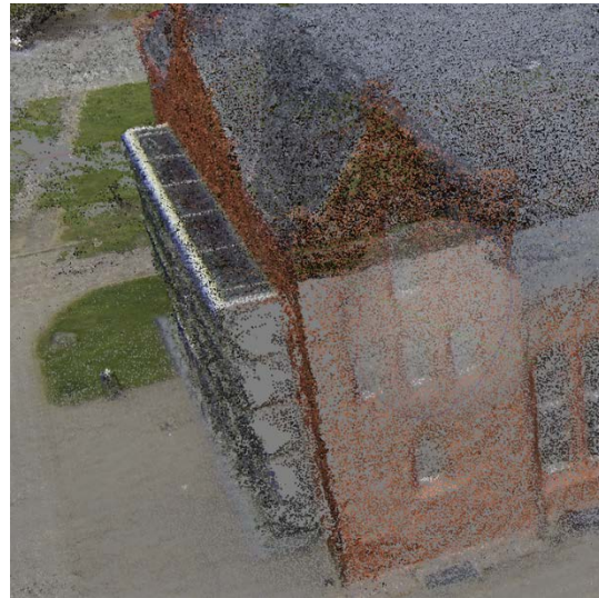
Figure 3. Dense Point Cloud, calibrated camera
