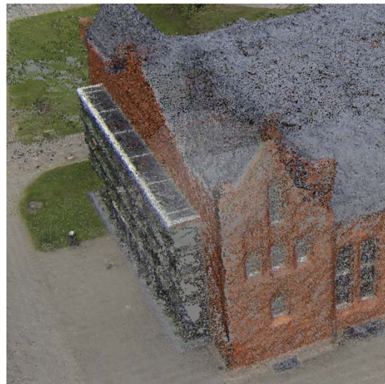
Figure 4. Dense Point Cloud, camera not calibrated
