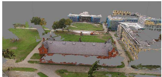
Figure 8. Reconstruction using 16 images (Dense Point Cloud)
