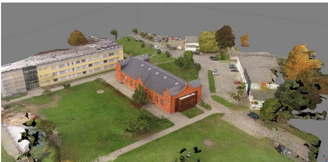
Figure 10. Reconstruction using 65 images, overview
