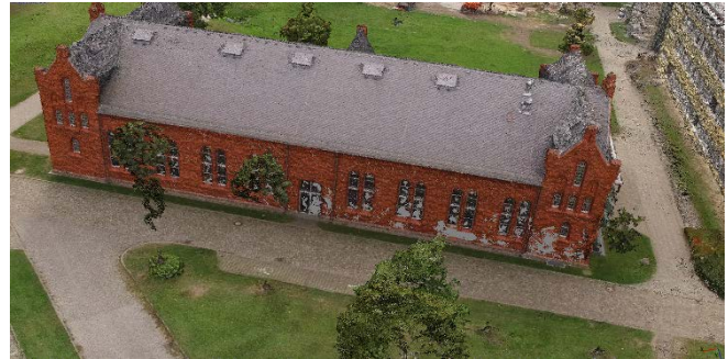
Figure 7. Reconstruction using 32 images (Dense Point Cloud)
