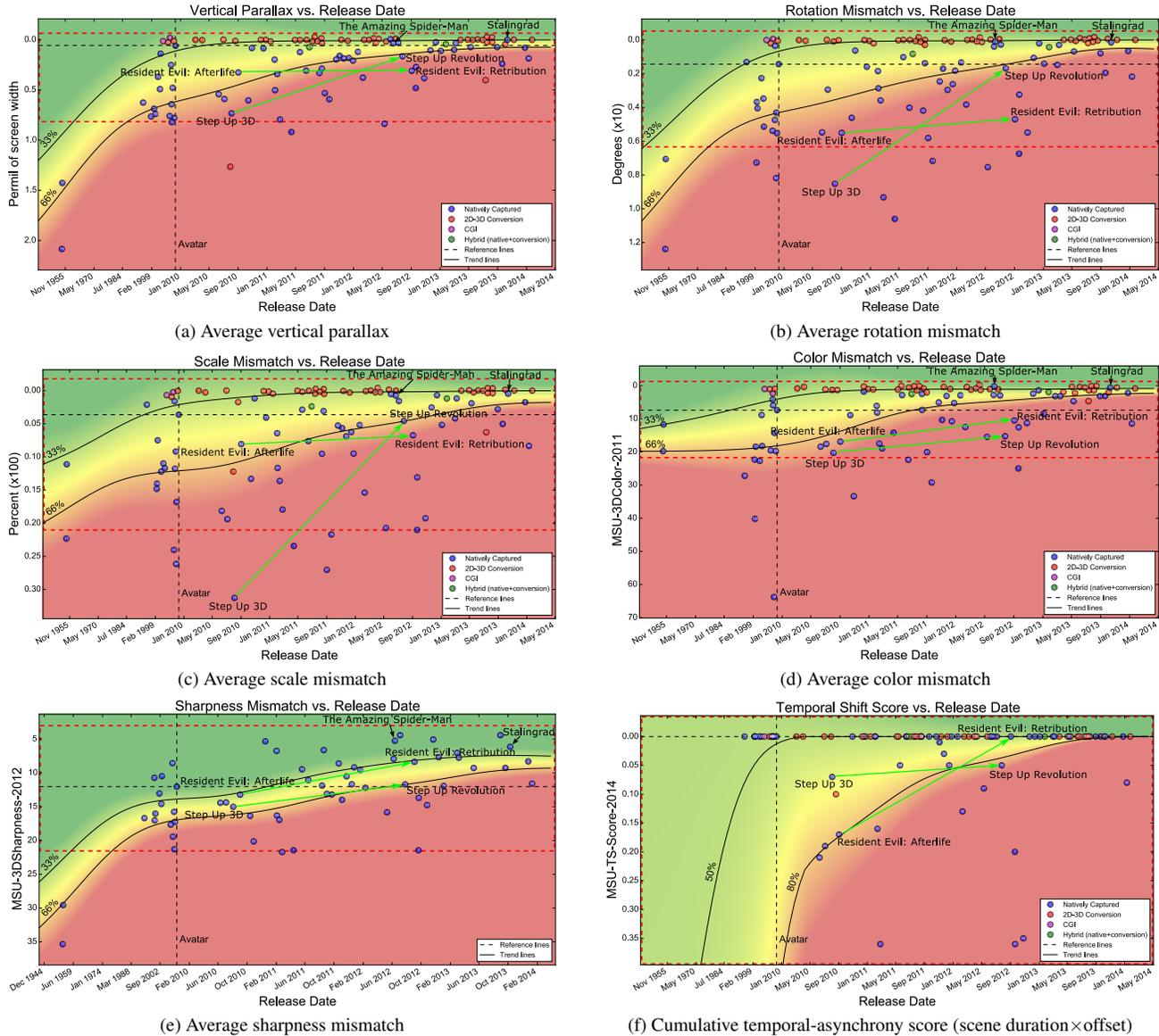
Figure 7: Results of common-S3D-artifact analysis depicting vertical parallax (a), rotation mismatch (b), scale mismatch (c), color mismatch (d), sharpness mismatch (e) and temporal asynchrony (f).
