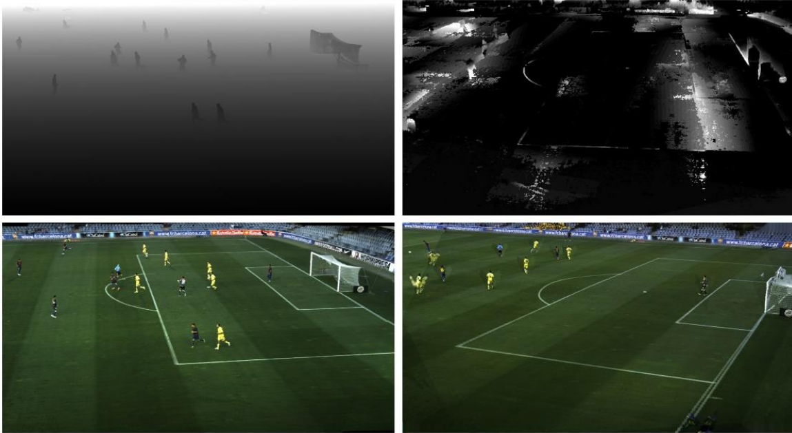
Figure 14. Depth Estimation (top) and View Synthesis results (bottom) with Segmentation-guided Plane Sweeping (left) and DERS/VSRS (right)
