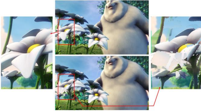
Figure 9. View synthesis with Depth-based view blending (left) vs. VSRS view blending (right)
