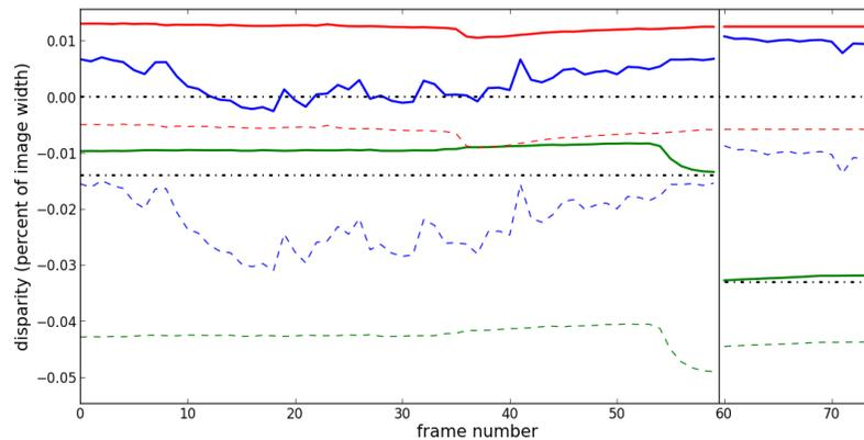
Figure 2: Linear depth mapping result of a short two-shot S3D video. Black dashed lines: screen (0.00) and minimum of comfort zone ( $-1.4$  first shot,  $-3.3$  second shot), thin dashed lines: minimum depth of frame (lower line), mean depth of object of interest (middle line), see e.g. figure 3), and maximum depth of frame (top line), solid lines: data of mapped video (order equal to dashed lines), vertical line: shot-cut.
