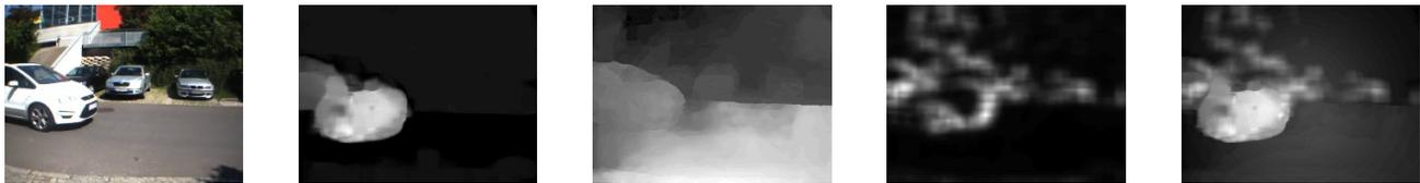
Figure 3: Saliency map computation of proposed S3D human visual attention model for multi-shot stereoscopic video analysed by figure 2. From left to right: left view of stereoscopic image, motion saliency map, disparity map, spectral residual saliency map and combined map based on maximum pooling and linear combination with center-bias.
