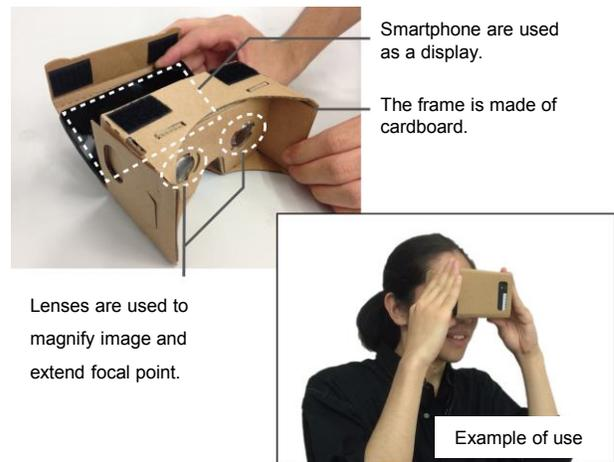
Figure 1. Simple frame HMD
