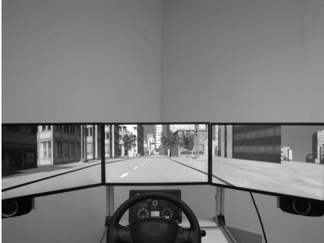
Figure 1. A view of the simulator in the first configuration, with 3 screens and a visual field on approximately 120 degrees. The supplementary screen behind the steering wheel is used as a dashboard in the simulator's original setup and was not used in the experiment to mask the car's speed.
