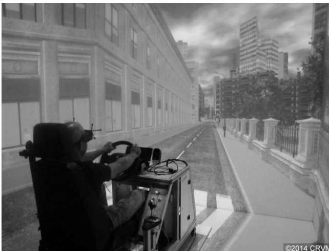
Figure 2. The simulator in the second configuration, installed in the CRVM's CAVE. This is a four sided setup, with a 10x10 inches floor and 3 vertical screens (10 x 13 inches), such that the whole driver's visual field was stimulated in that configuration.
