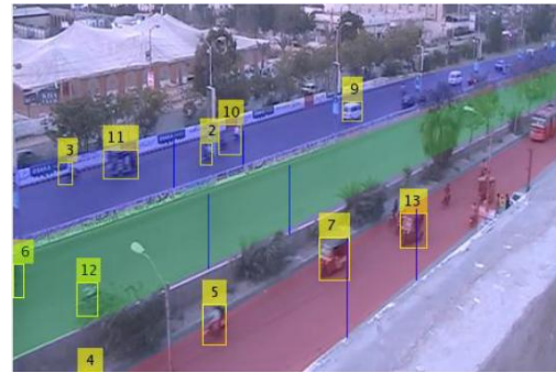
Figure 3: Implemented detector results. Registration lines are shown in blue color for each lane.
