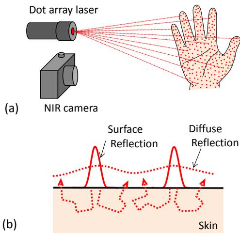
Figure 1. Alice System. (a) schematic illustration of the system; (b) surface and diffuse reflectance from skin.
