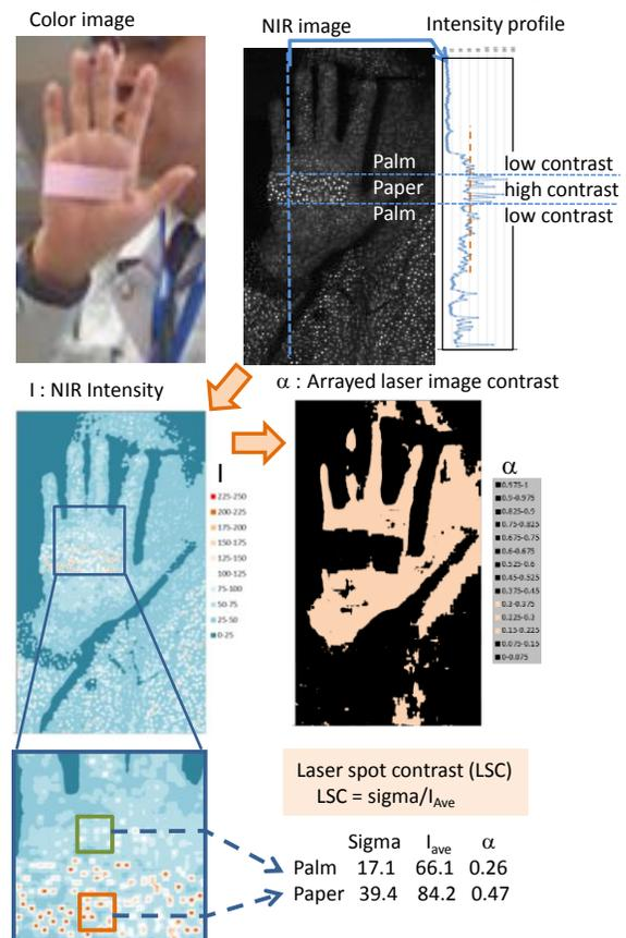
Figure 3. Alice data processing for human body detection. In this case, LSC ( $\alpha$ ) was calculated in 7x7 pixel frames. Hand and face were successfully detected through image processing.
