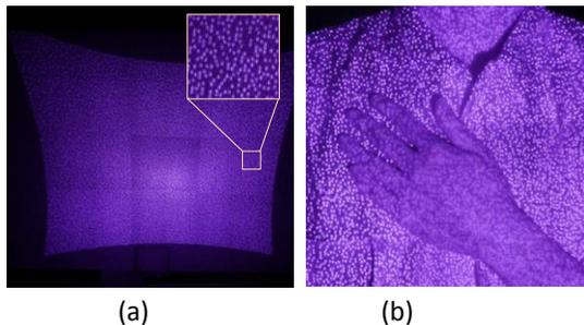
Figure 2. Projected dot array pattern. (a) NIR image projected on a wall, (b) NIR image of hand on cloth.
