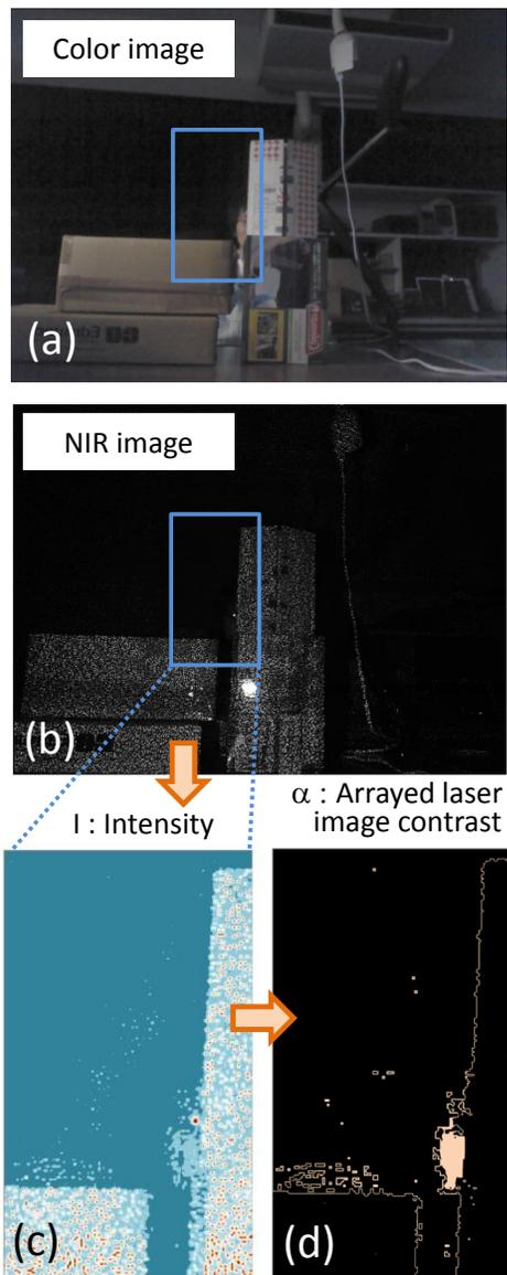
Figure 6. Detection of occluded human body. A person hiding behind boxes could be detected.
