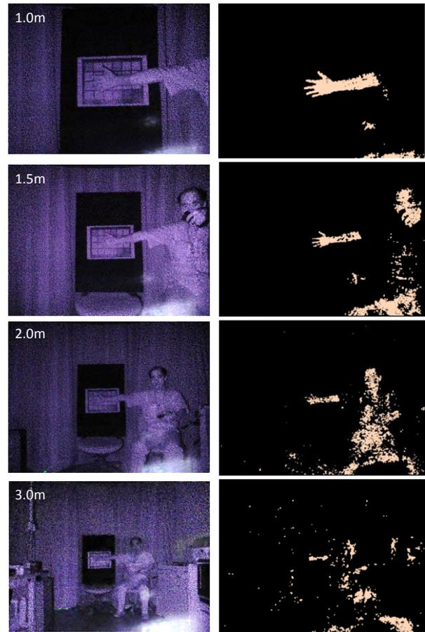
Figure 4. Human body detection performance of the Alice system as a function of distance between target and camera.
