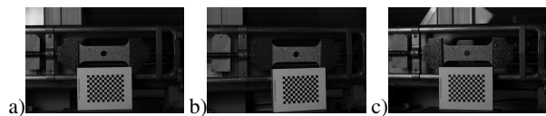
Figure 8. Example series of images used to reconstruct shape of a measured object: a) image captured from the front, b) image captured at -15^\circ , c) image captured at +15^\circ .
