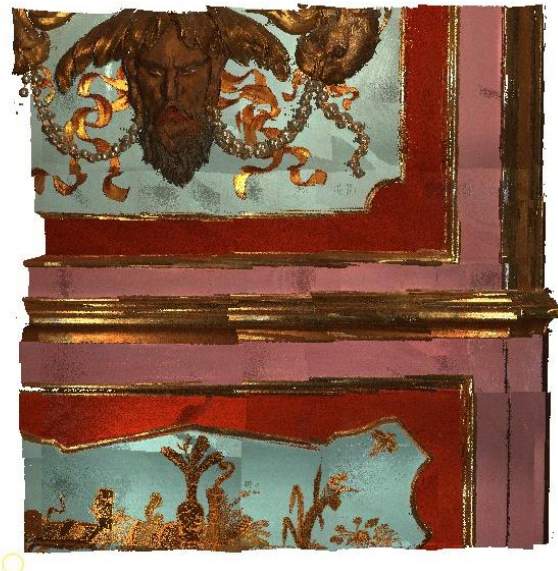
Figure 11. Visualization of misalignments between directional clouds of points.
