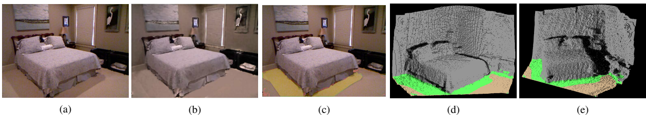
Figure 9: Sample comparison between the shadow removal result in [3] and the shadow detection result of our method. (a) original bedroom scene (b) shadow removal result in [3] (c) our result compared with our manual label (d) our result in point cloud, front view. (e) our result in point cloud, side view. In (d) and (e) green area indicates detected shadow.
