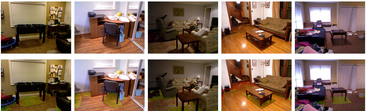
Figure 8: Shadow detection results on part of NYU Depth Dataset. In the bottom row, red mask indicates detected shadow, green mask indicates manually labeled shadow yellow mask indicates agreement.
