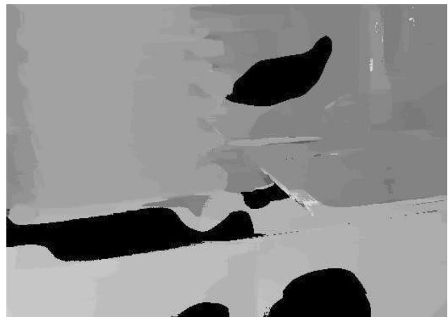
Figure 2. Input: Original disparity map D(x,y) (black areas are disparity holes)
