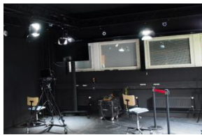
Figure 23. Motion capture studio, the blue rings are the IR cameras.
