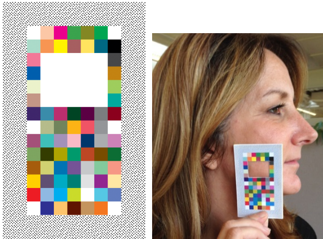
Figure 2. The StegaFrame enclosed color calibration target and its use for capturing a skin tone sample.
