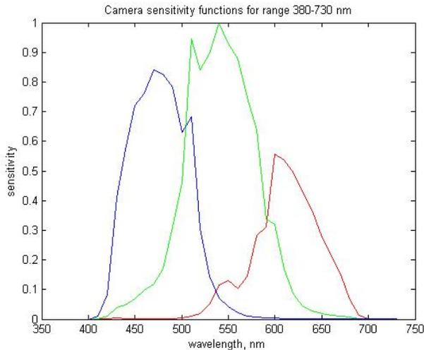
Figure 1. Sensitivity function of the camera model used in simulations.
