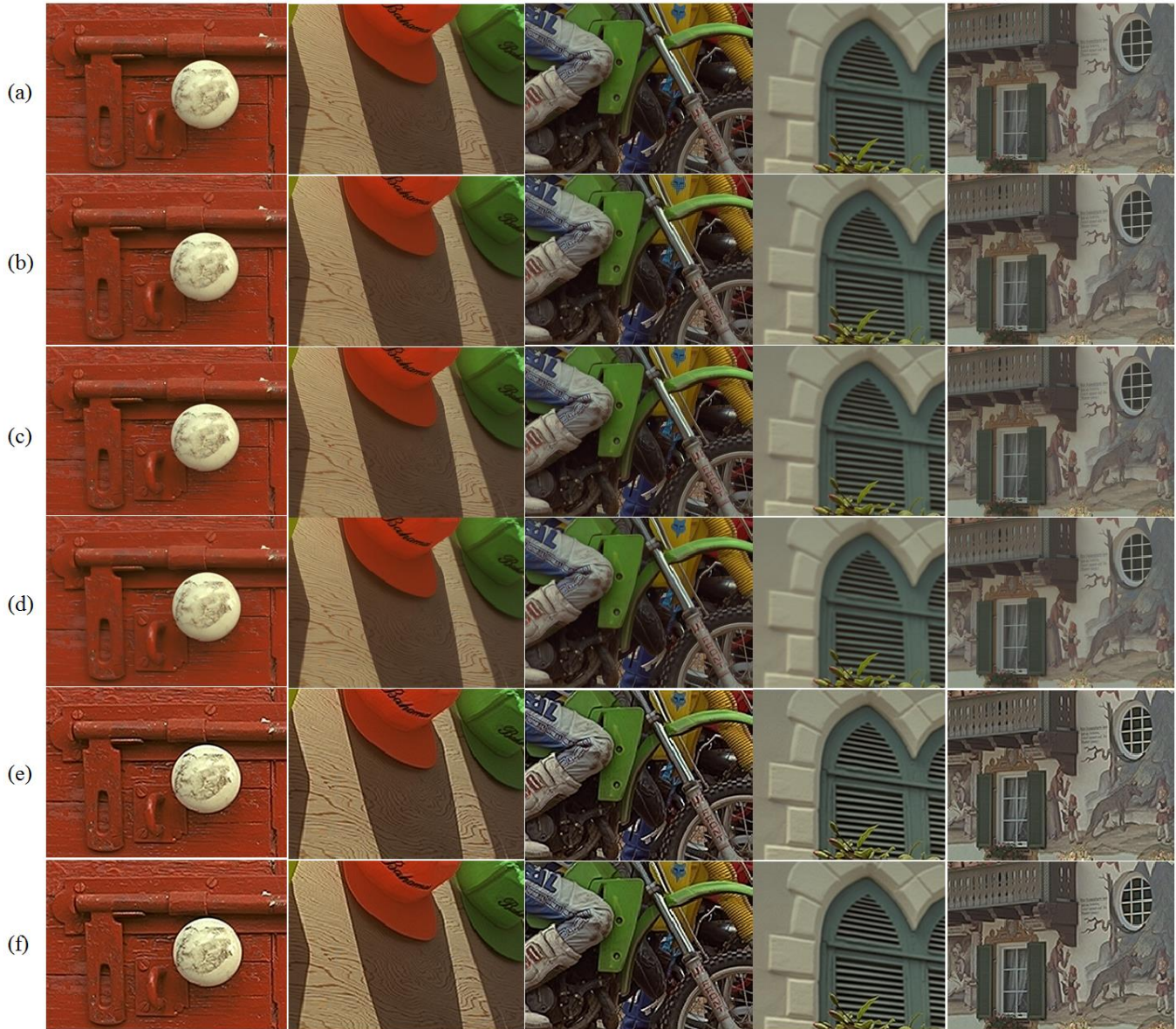
Figure 5. Portion of five different Kodak PhotoCD benchmark images, no. 2, 3, 5, 7, and 24: (a) original image, (b) iterative demosaicking using weighted-edge and color-difference (IDWC), (c) alternating projection (AP), (d) nonlocal adaptive thresholding (NAT), (e) proposed method with Bayesian classifier, and (f) proposed method with SVM classifier. Proposed methods provide better detail texture or pattern of rigid objects and structures in demosaicked images.
