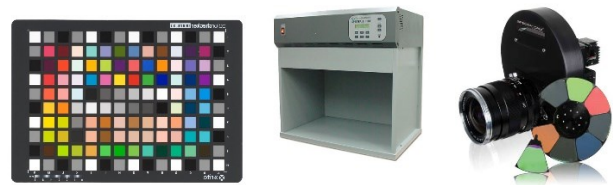
Figure 1. From left to right: the X-rite Colorchecker SG chart, the Macbeth Spectra Light III light booth and the Pixelteq SpectroCam VIS-NIR.
