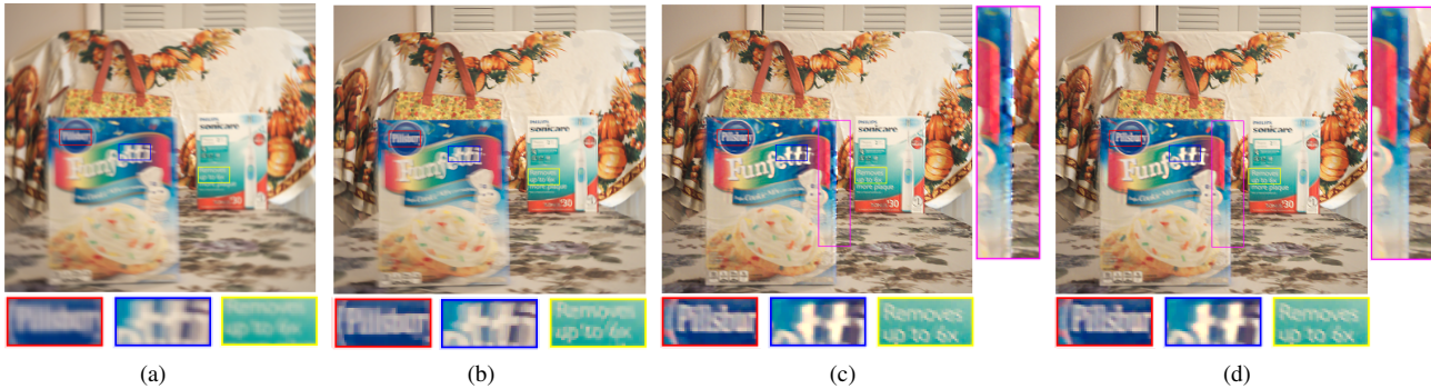
Figure 5. Depth-aware motion deblurring on a real image with large depth variation (a) blurred image (b) deblurring result of [20] (c) our restored image using Projective Motion Richardson-Lucy algorithm (d) final restored image using modified Richardson-Lucy algorithm
