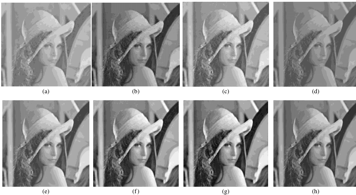
Figure 2. Reconstructed "Lenna" image at the lowest subrate of 0.1 (highest CS ratio) for the original algorithms: (a) BCS-SPL-DWT, (b) BCS-SPL-DCT, (c) BCS-SPL-CT, and (d) BCS-SPL-DDWT, and for the enhanced algorithms: (e) GM-BCS-SPL-DWT, (f) GM-BCS-SPL-DCT, (g) GM-BCS-SPL-CT, and (h) GM-BCS-SPL-DDWT.
