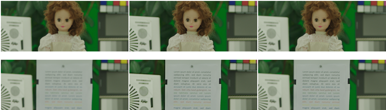
(a) The blurred input image (b) Applying global deblurring method (c) Deblurring only applied in the region of interest Figure 14: Depth selective image deblurring applied on the test shots Doll and TextScene by only deblurring the object of interest while leaving the background unprocessed (SLD). Selecting the interval, deblurring is applied in, is guided by the captured depth map. The doll is located 14 cm in front of the focus. The text plane is located 20 cm in front of the focus. The used selected method is SAP.
