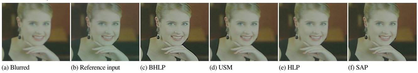
Figure 8: Visual comparison of non-blind and blind deblurring approaches for the shot 'WomanPlane' at 190cm (best viewed in electronic version. Zoom for more details)
