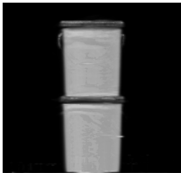
Figure 4. 2-D projection of reconstructed 3-D water bucket volume
