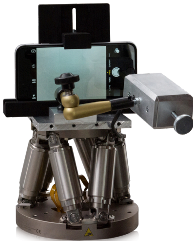
Figure 11. The hardware apparatus with the DUT. The hardware allows a movement with six degrees of freedom, so pitch, yaw, roll and translation in X, Y, Z direction. The device shakes the camera with the standard handshake as published by CIPA. The mobile phone camera is mounted that way, that it can capture images of the test chart. The image shows a mechanical "finger" that can be triggered from control software to press the release button. In the final measurement, this was replaced by a smaller solution that can trigger the touch button directly.
