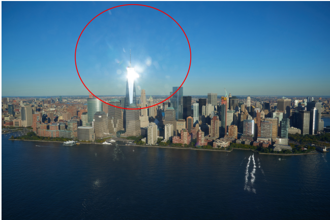
Figure 1: around the specular highlight ghosting artifacts are visible due to reflections on surfaces within the lens.
