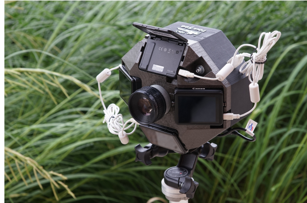
Figure 2. FourSee multi-camera TDCI prototype
