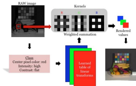
**Figure 1.** Overview of the  $L^3$  processing pipeline. Class specific linear transforms are precomputed and stored in a table. Each captured sensor pixel is classified into one of many possible classes, and the appropriate linear transform is applied to the pixel and its neighborhood to render the data
