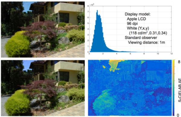
**Figure 2.** Comparison between camera RGB (upper left) and  $L^3$  RGB rendered with local linear filters (lower left). The image at the lower right shows the S-CIELAB  $\Delta E_{ab}$  values for each pixel. The histogram of errors is shown on the upper right. The mean error is 1.59, the peak error is near 8, and the standard deviation of the  $\Delta E_{ab}$  values is 0.9. These errors are typical for the 11 images in the independent test set.
