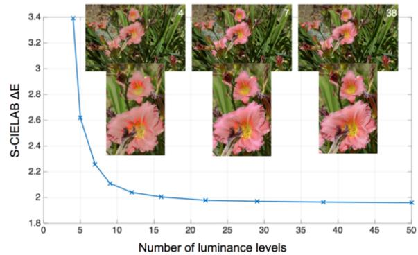
**Figure 3.** The selection of classes can have a large impact on the quality of rendered images. This graph shows images rendered with a small, medium, and large number of response level classes. In all cases the response levels are separated logarithmically. The flower (zoomed view) changes substantially as the number of levels increases, and the mean rendering error declines significantly as the number of classes increases from 4 to 15.
