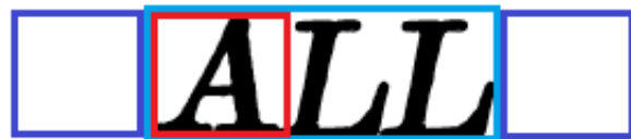
Figure 5. The blue rectangle is minimum enclosing box of label “All”, the red rectangle is minimum enclosing box of character “A”, and the purple rectangles are potential character areas.
