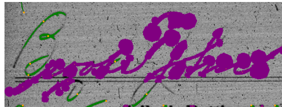
(c) Previously visited pixels (purple) are ignored on the second pass. New start points (orange) are chosen using the unvisited connected components (green)
