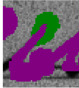
Figure 10: A wavefront at the end of a stroke (green) expands in a circle and is pruned.
