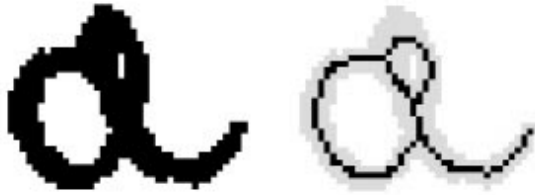
Figure 2: An example of a handwritten lower-case ‘a’ and its skeleton, obtained by line thinning. Taken from a figure in the paper by L’Homer [10].
