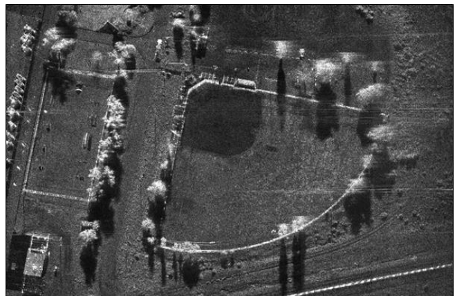
Figure 1. Synthetic Aperture Radar (SAR) image of a baseball diamond. Image courtesy of Sandia National Laboratories, Airborne ISR.
