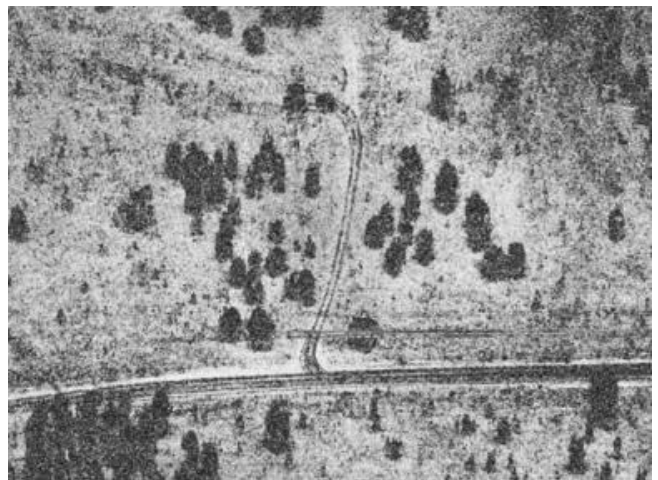
Figure 2. Coherent Change Detection (CCD) image highlighting several changes between images taken of the same scene at two different times. Image courtesy of Sandia National Laboratories, Airborne ISR.
