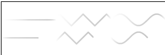
Figure 4. Path Deformations (left to right): straight, angular, wavy
