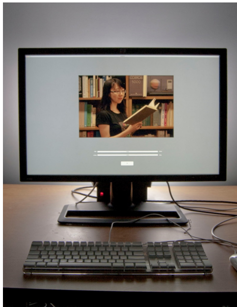
Figure 7. The experimental setup. The room is dark except for the rear wall, which is lit with a light positioned behind the display.
