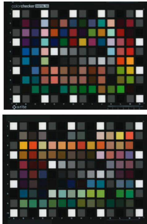
Figure 2: Comparison images of the SG (top) and SGX (bottom) targets
