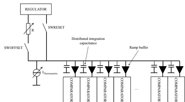
Figure 7: Schematic of the I/C ramp generator.
