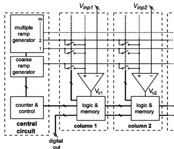
Figure 3: Architecture of the MRMS technique.
