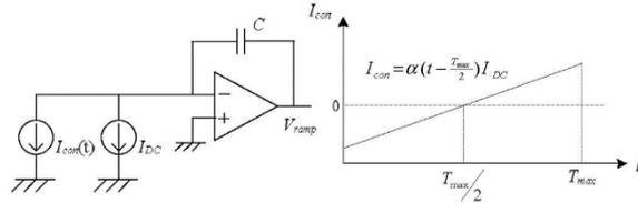
Figure 12: schematic of a nonlinear ramp.
