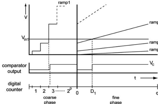
Figure 5: Timing for the Multiple Ramp Multiple Slope ADC.
