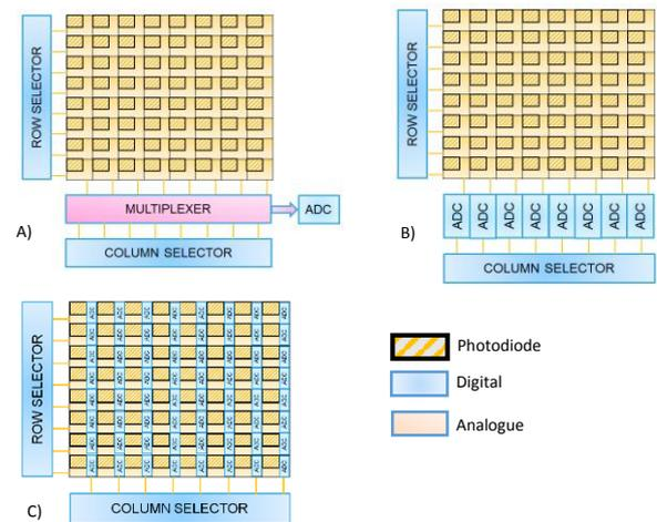
Figure 1: Several architectures to increase readout speed.
