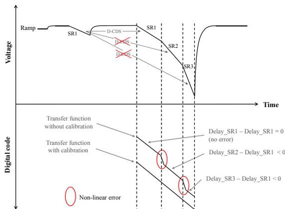
Figure 9: Conversion errors introduced during the conversion.
