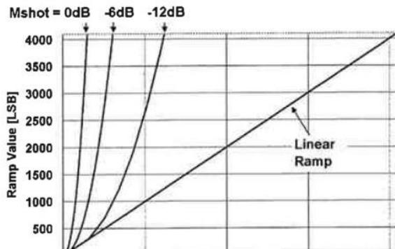
Figure 13: Timing of the nonlinear ramp for different margin [11].
