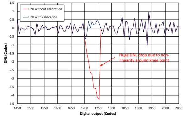
Figure 10: DNL before and after calibration.
