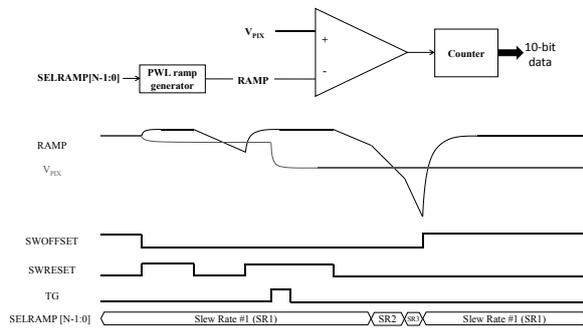
Figure 8: Timing diagram of the Piece wise linear ramp generator
