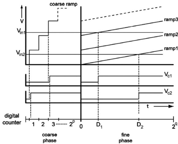
Figure 4: Timing for the Multiple Ramp Single Slope ADC.
