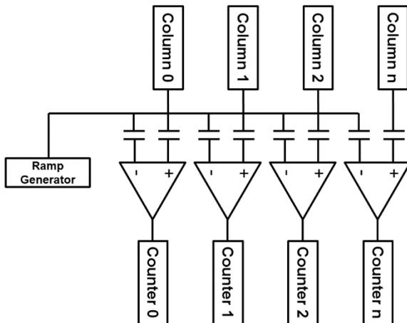
Figure 2: Column parallel SS-ADC architecture.
