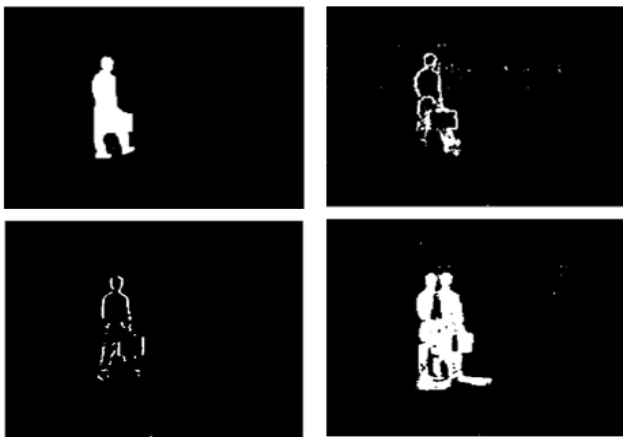
Figure 4: From left to right and up to down A- Ground truth of the moving object given in the dataset B- Movement detected for a quantization of 8bits with the first algorithm C- Movement detected for a quantization of 3bits with the first algorithm D- Movement detected for a quantization of 8bits and framerate divided by 9.
