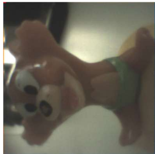
Figure 8. Capture image of the NanEye camera using mathematical gamma function of 1.2
