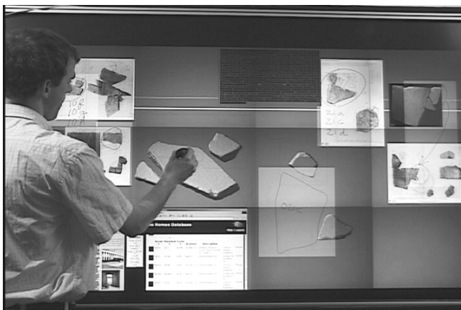
Figure 1: A 4x3 projection array, the Stanford Interactive Mural. Displayed are images, sketches, 3D models and a virtual desktop. The user interacts with the content using an eBeam pen
