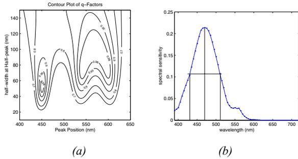
Figure 3. (a) Preferred peak Positions and half-width; (b) Estimating the half-maximum width for any spectral sensitivity functions with single primary peak
