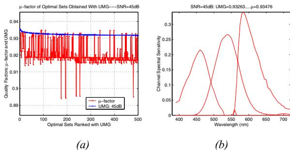
Figure 6. (a)  $\mu$ -Factor of 500 optimal filter sets obtained with UMG; (b) The optimal set with maximal UMG value
