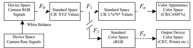
Figure 1. Processing pipeline of digital camera signal, where  $F_s$  are transformations
