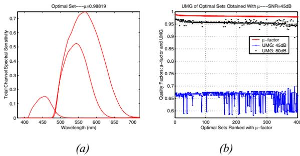
Figure 4. (a) The "optimal" sensitivity function set obtained with  $\mu$ -factor, shape is not optimal; (b) the UMG and  $\mu$ -factor values of the 400 "optimal" sets
