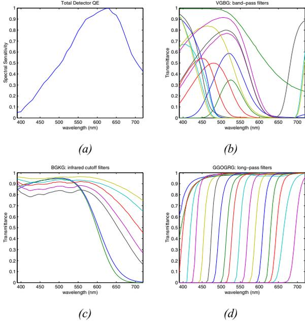
Figure 2. (a) CCD QE curve; (b) Transmittance spectra of bandpass filter elements; (c) Transmittance of infrared filter elements (d) Transmittance of longpass cutoff filter elements
