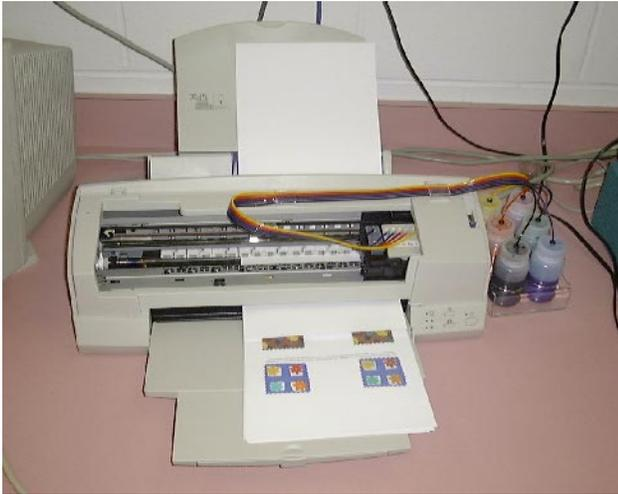
Figure 9. Epson 1200 retrofitted for continuous 6-ink feeding
