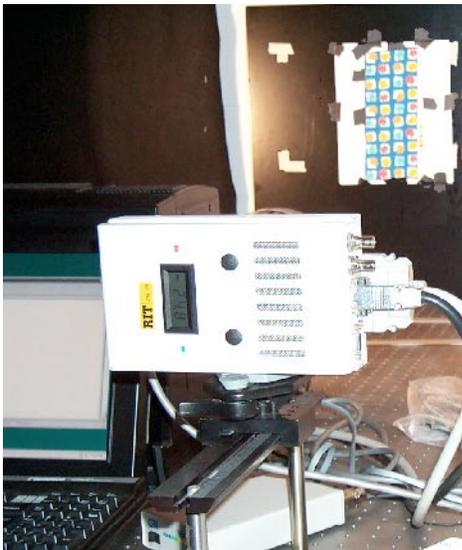
Figure 3. Photometrics Quantix camera (foreground) imaging *Brite Lites* fabric (background). Lens and CRI tunable filter (not visible) mounted in front of camera. Also out of view for this illustration are Bogen quartz lamps to the left and right.
