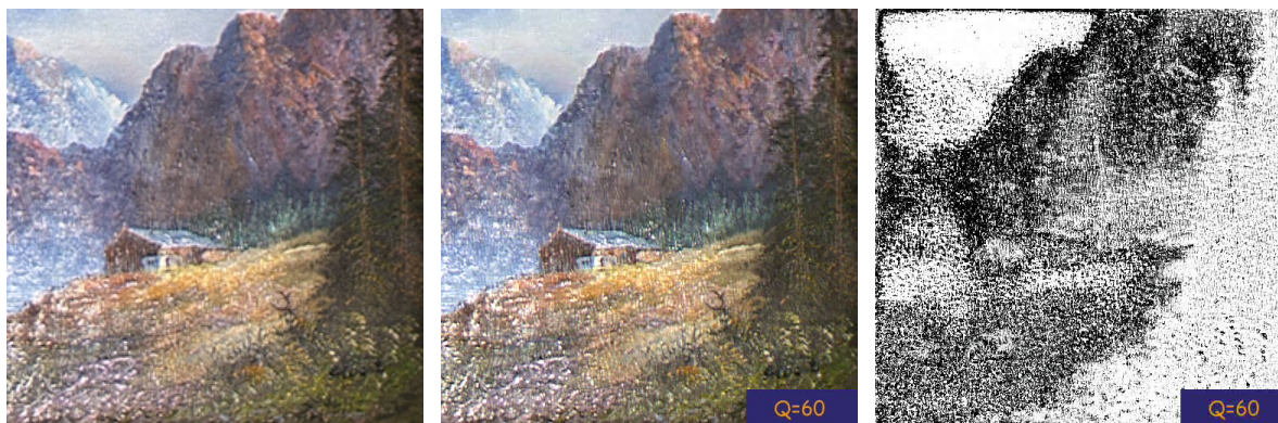
Figure 9. Example of distortion map, (a) original image, (b) compressed image, (c) distortion map
