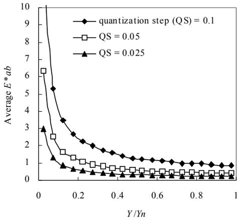
Figure 2. The average  $E_{ab}^*$  caused by linear quantization of WKL coefficients over normalized  $Y$ .
