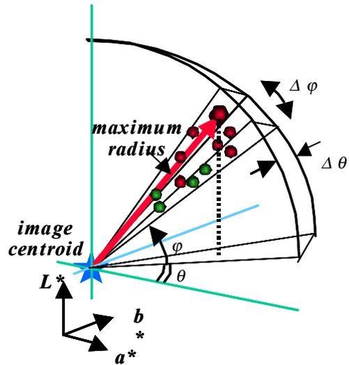
Figure 1. Segmentation of image gamut in Polar coordinate
