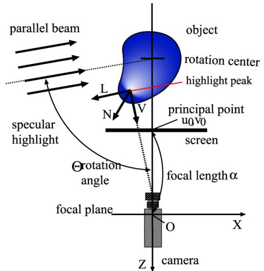
Figure 5. Model for measuring a specular highlight
