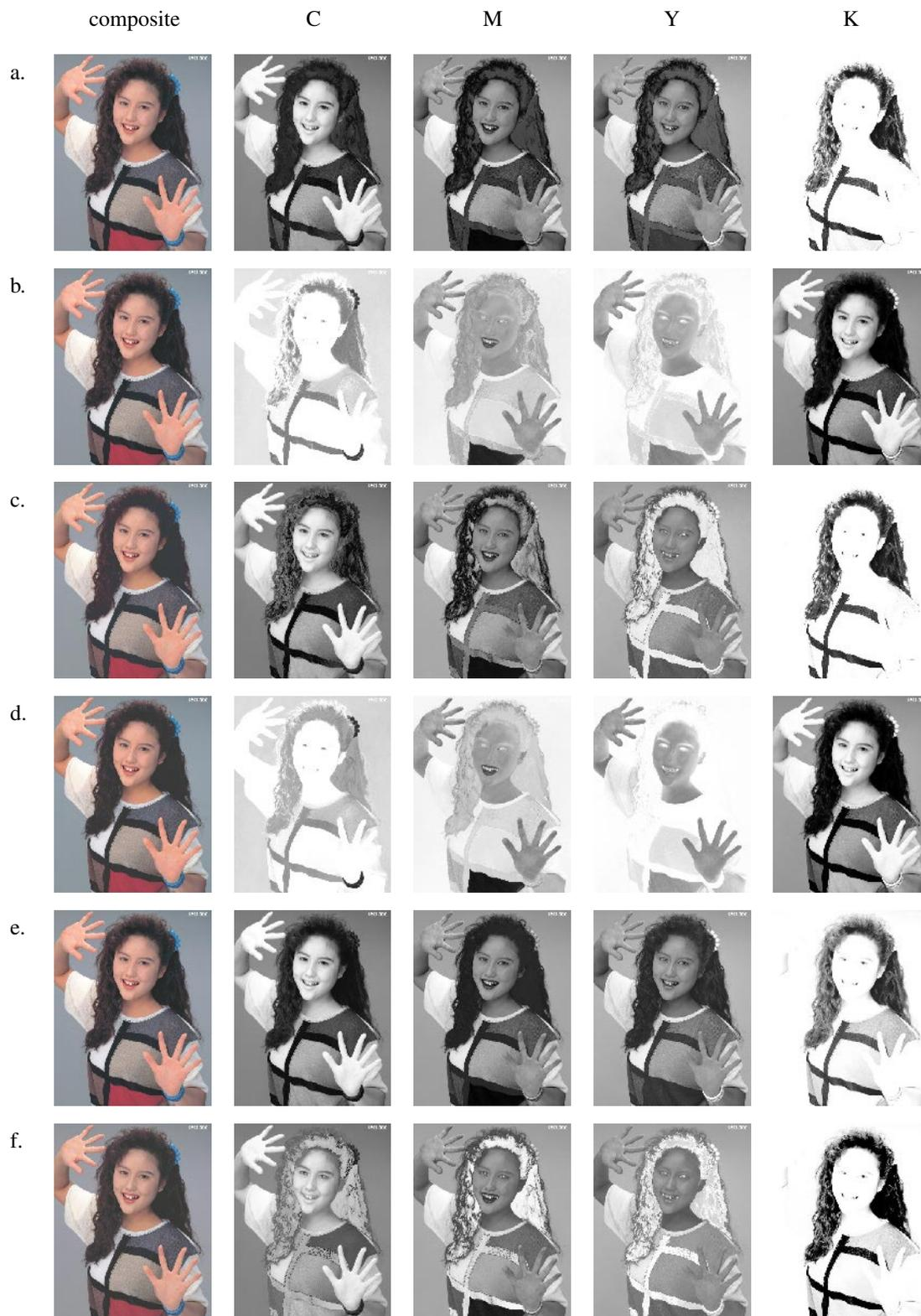
Figure 3: Separations of the SCID image N1 assuming SWOP colorants: a. SWOP  $K_{MIN}$ ; b. SWOP  $K_{MAX}$ ; c. target printer  $K_{MIN}$ ; d. target printer  $K_{MAX}$ ; e. original CMYK separations; f. target printer using proposed method. The columns two to five are CMYK separations and the first column is the resulting composite image.
