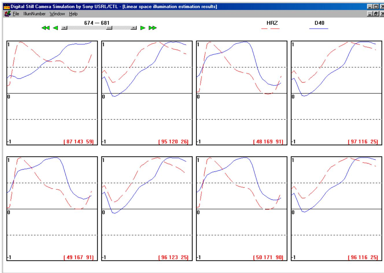
Figure 3. Surface reflectance computation for different illumination hypotheses. The actual illumination is Horizon.
