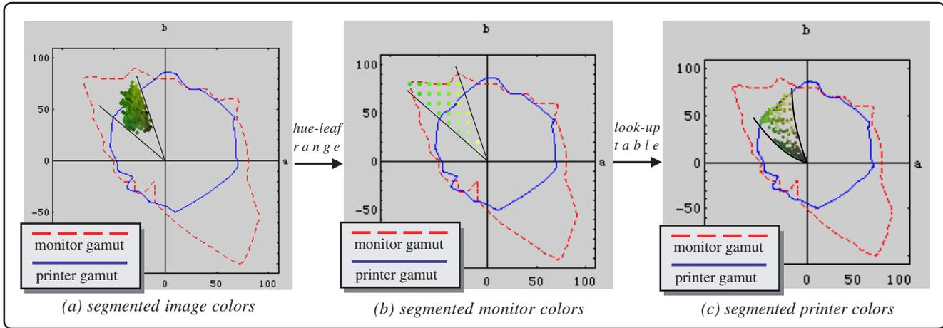
Figure 4 The hue-leaves of segmented image and devices. The hue-shift problem occurring in segmented printer colors is solved by using look-up table.
