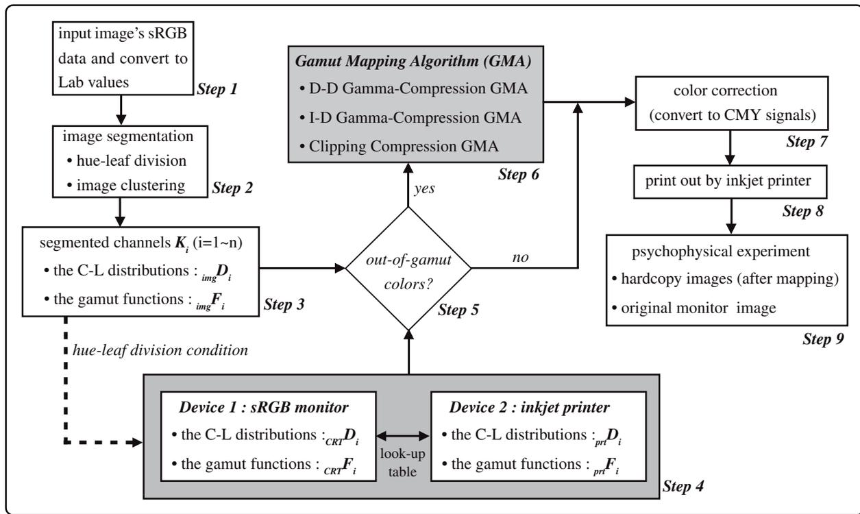
Figure 2 Flow diagram of gamut mapping process.
