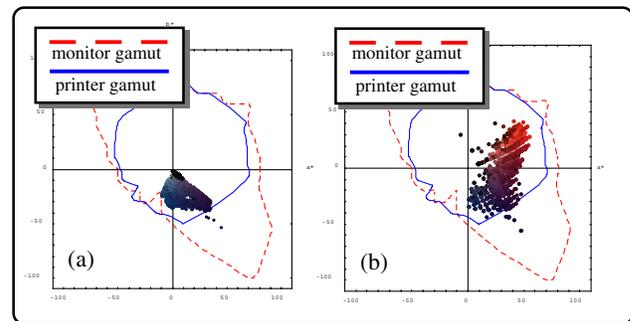
Figure 8 The natural image channels having out-of-gamut blue colors segmented by (a) hue-leaf division, and (b) image clustering.
