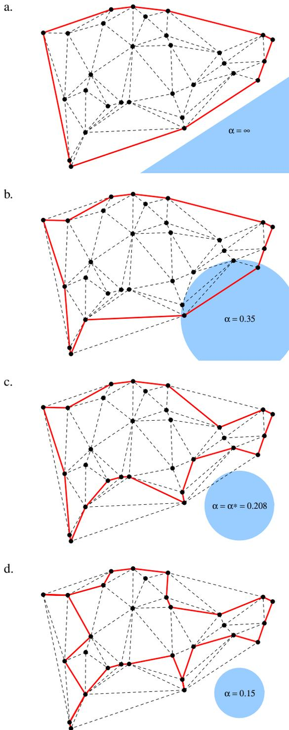
Figure 1: A family of two-dimensional alpha-shapes for different values of  $\alpha$ . Dashed lines show the Delaunay triangulation of the set of points and a thick line is the edge component of its alpha-shape. The disk in the right corner has radius  $\alpha$ . The first alpha-shape ( $\alpha = \infty$ ) is identical to convex hull and the disk is a half-plane.
