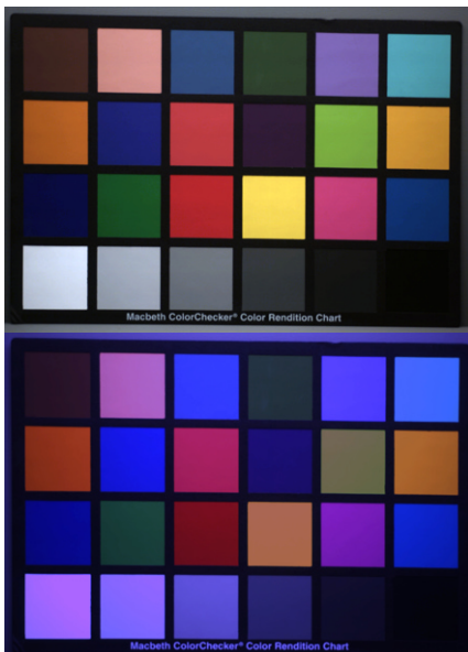
Figure 7. Macbeth Checker Chart under Illuminant A and TL84 corrected for D65 using grey-world algorithm.
