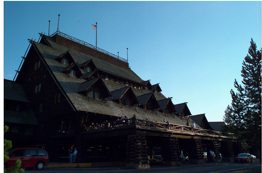
Plate 2a: A photographic reproduction model is used to capture a high dynamic range scene. Shadows are blocked up in the reproduction because the model assumes a scene dynamic range of 160:1, and this scene is 1400:1.
