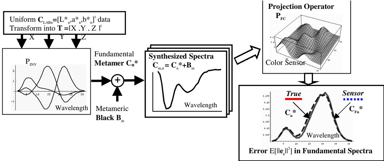
Figure 2. Flow diagram for testing the spectral response errors in color sensors
