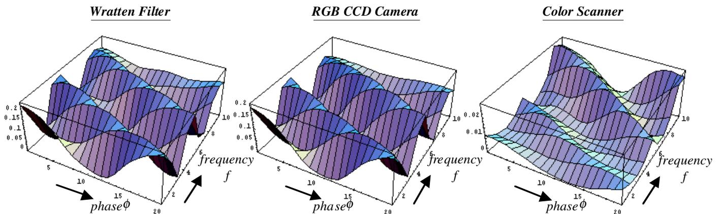
Figure 7 (b). Changes in spectral response errors vs.  $(f, \phi)$  of metameric black sources **B2**( sine SPDs)
