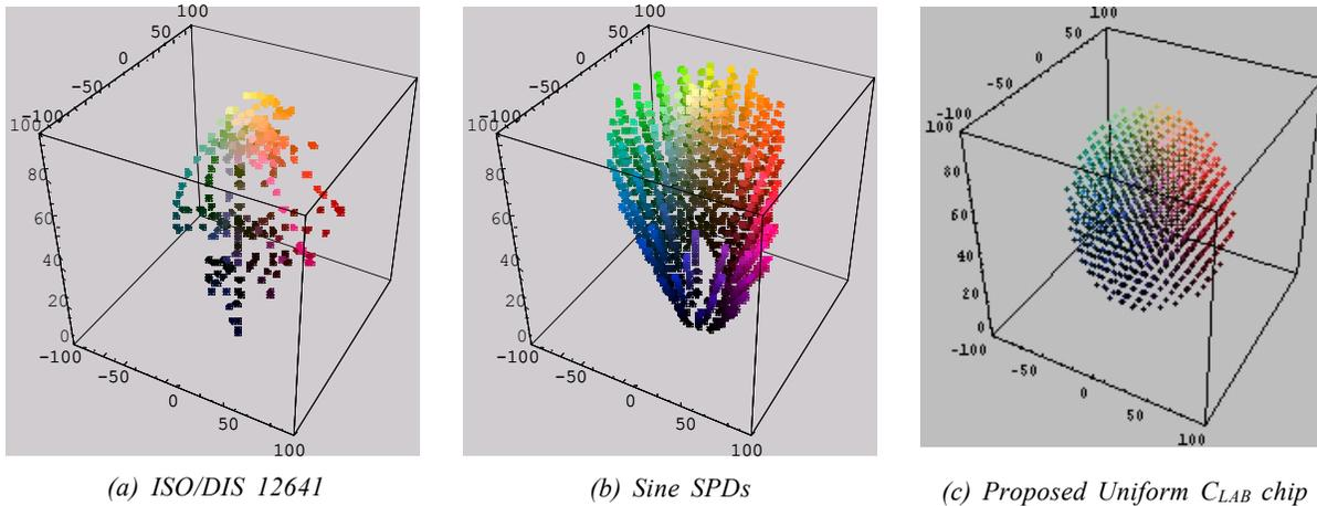
Figure 1. Color distributions of test chips in CIELAB space
