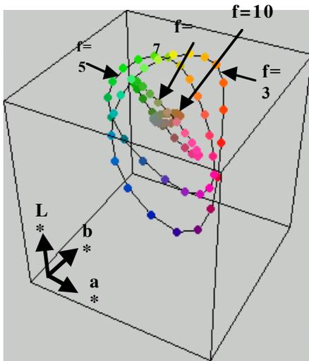
Figure 3. Spectral loci of sine SPDs vs. frequency  $f$
