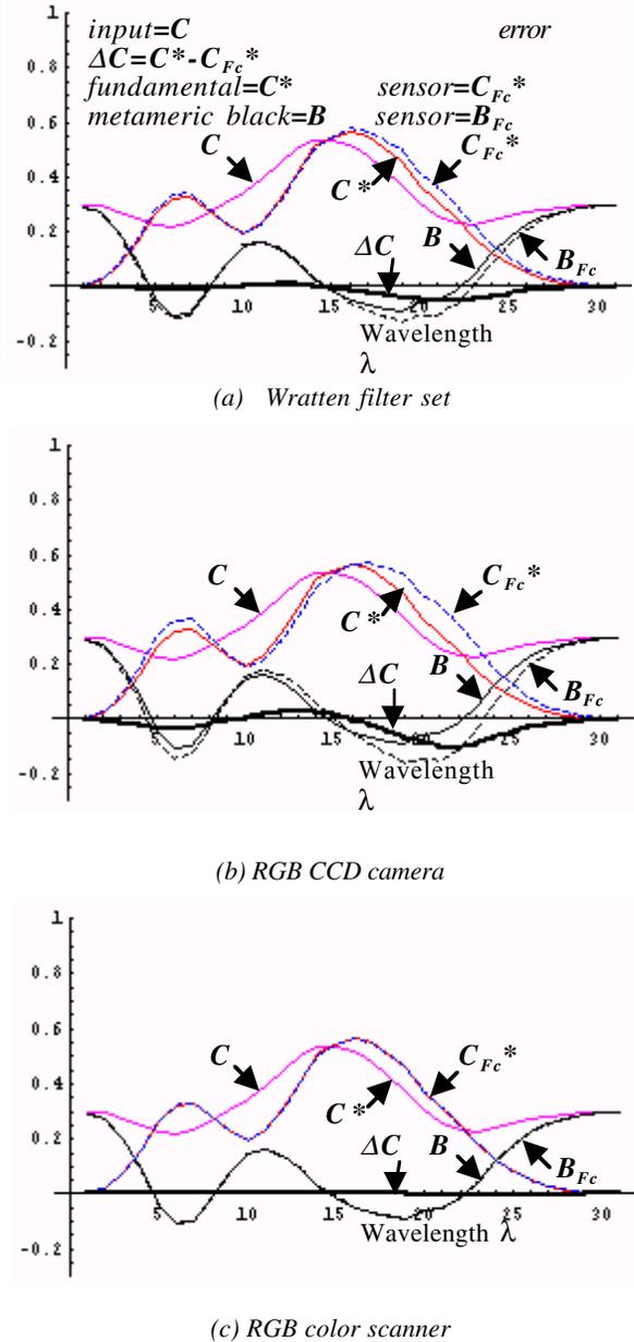
Figure 6. Spectral response errors in tested color sensors
